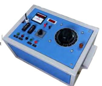
The primary injection kit has different models with range of output currents from 100A to 1500A. These are well protected with the provision of MCB against OVERLOAD than the rated current. HRC fuse protection is provided for control circuits.
