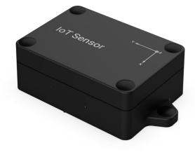
KL310-TILTisaLoRaWAN ® tilt sensor mainly for angle measurement and asset movement detection. With a compact size and 3-axis accelerometer, KL310-TILT can be installed to the objects easily to measure its X, Y, Z tilt angles. It can also detect the movement based on angle change sand send threshold alarms. Compliant with KLED LoRaWAN® gateway and KLED IoT Cloud solution, users can know the angles and tilt threshold alarms in real-time via browser or mobile app remotely.
