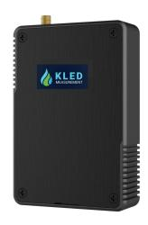
KL56 is a robust 8-channel indoor LoRaWAN gateway. Adopting SX1302 chip and high-performance quad-core CPU, KL56 supports connection with more than 2000 nodes. KL56 has line of sight up to 15 km and can cover about 2 km in urbanized environment, which is ideally suited to smart building, smart industries and many other indoor applications.
