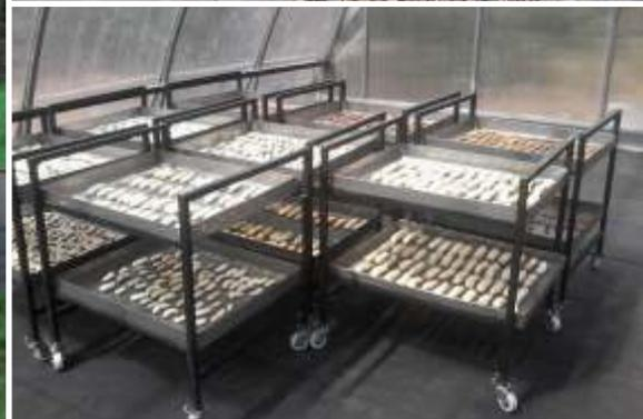
SUNLIT Solar tunnel Drier is an enclosed chamber which is used for drying of various crops using Green House effect. It helps to preserve the food and also increase the shelf life of the product. It is covered with multi layer Polycarbonate sheet which traps solar energy and has an insulation effect, thereby maintaining high temperature for a longer period of time. Further solar tunnel drier filters out the UV radiations which help products to retain the nutrients, hygiene and colour.
