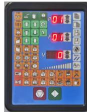
The A-series wrapping machines are equipped with the EasyOP. An extensive control panel including all basic functions of the FS380 and FS500. It is installed in a separate control cabinet attached to the mast.
