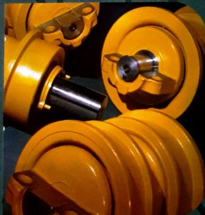
Steel forged deep hardened on the rail surface insures the ultimate resistance to wear with maximum roller life. Double self align spherical bearing housed with L- blocked wheel assemblies
