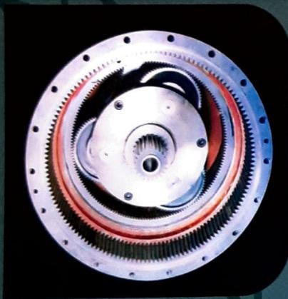
Planetary gear units for main hoisting specially design to fit inside the rope drum & acquires minimum space for crab trolley
