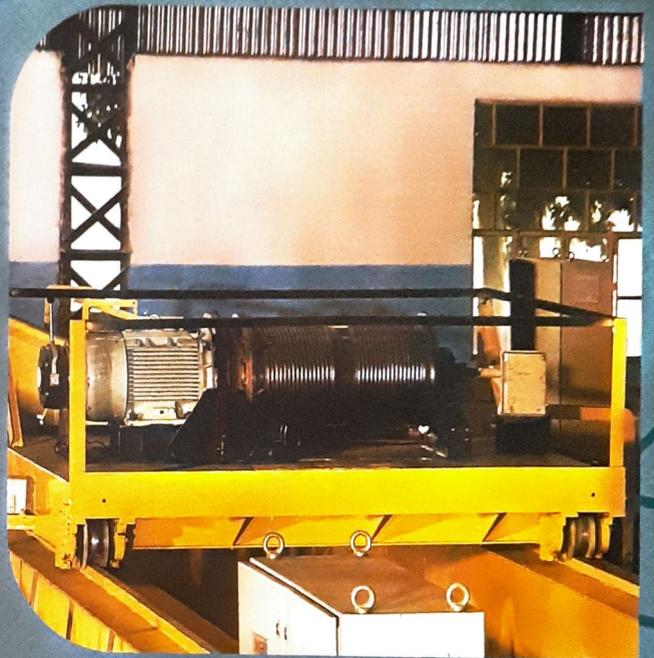
**Rope Drum :** It is made of steel on which wire rope grooves are accurately machined for proper sitting of wire Rope. Specially designed arrangement is provided so that Wire Rope changing is very easy without involving any clamping or tightening on the drum.
