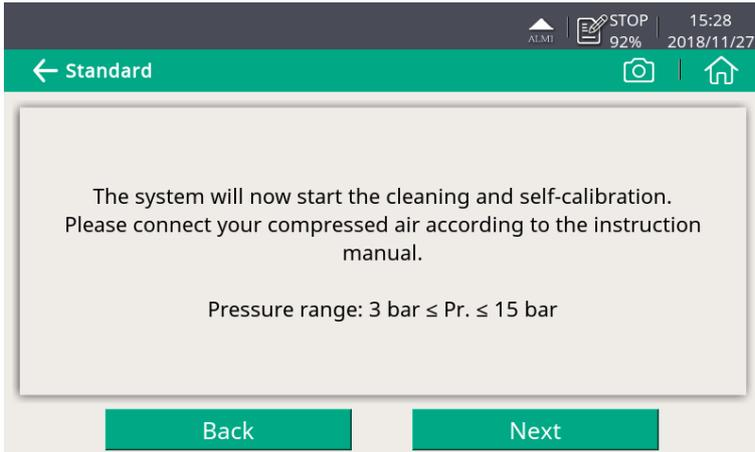
7. The system checks whether the pressure is in the valid range.
