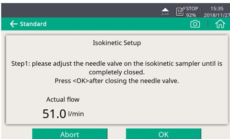
3. Perform Isokinetic setup as instructed on the screen.
