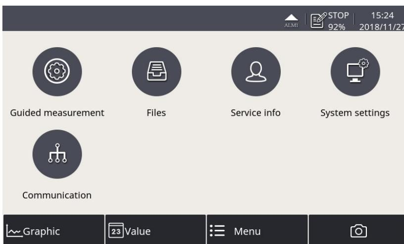
Access the main menu by clicking Menu in the bottom bar. The screen with sub-menus is shown.
