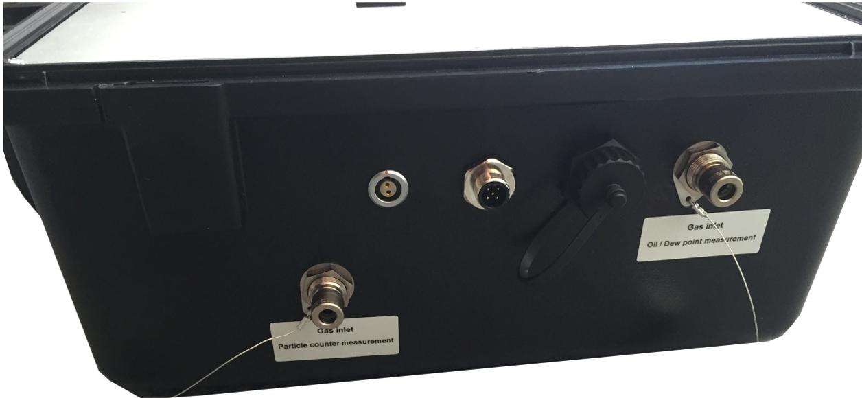
The S 600 offers two compressed air inputs on the right side of the housing. The inlets are shown on the picture above and are marked respectively to their functions: *Gas inlet Oil / Dew point measurement* and *Gas inlet Particle measurement*.
