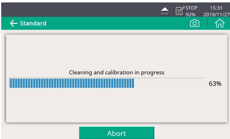
8. The system performs the self-calibration cycles and cleans the internal sensor components.
