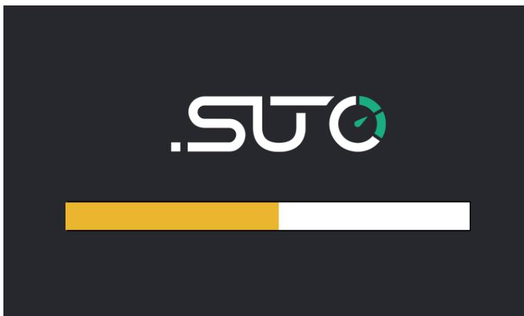
After the S 600 gets powered, the initialization screen is displayed with an active progress bar.
