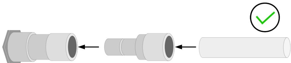
Directly plugging and pulling the teflon hose more than once may lead to particle contamination, which can affect the measurement. To avoid this problem, please use the included adapter plugs and keep them on your tubes.
