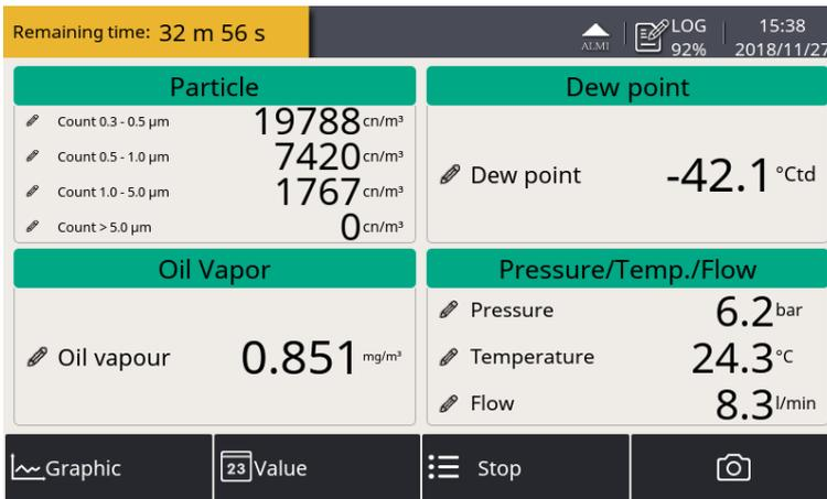
During the measurement, you can see the Data logger status icon on the status bar switched from STOP to LOG. The remaining time is displayed in the upper left corner. Please wait. The system will stop the measurement automatically.
