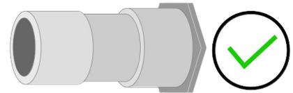
Remove the protection caps from all parts of both sides of the instrument. If not removed, the device may get damaged and the risk of bursting parts under high pressure can even lead to personal injuries. All exhaust outlets will pass air during the measurement, if not, please contact the manufacturer.
