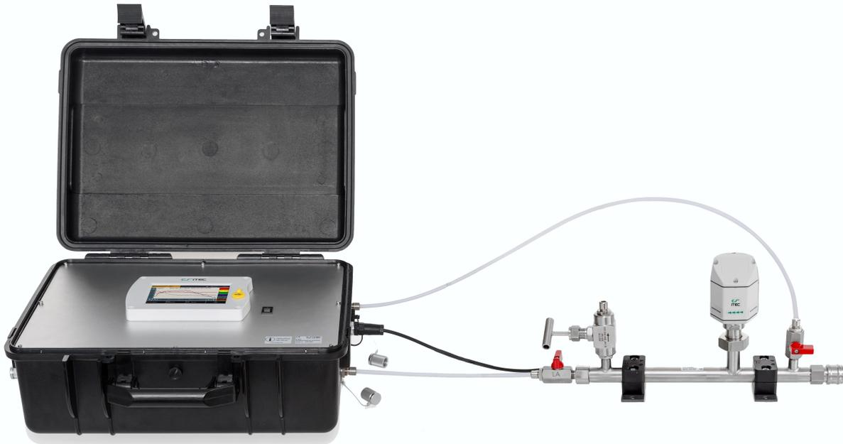
The picture above shows the S 600 setup with the isokinetic sampling device connected. Please connect the isokinetic sampling device using the teflon hose delivered with the device. On the next page you can find the detailed description of the sampling device. Also you can find which outlets of the sampling device need to be connected to which input at the S 600.
