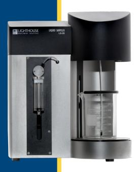
HE LS-20 Liquid Sampler has an integrated syring sampler and optical particle counting system. It's eas-to-use Windows<sup>tm</sup> based software interface is designe dto meet the intertnational reglatory EP and JP, as well as USP 788 requirements.
