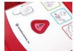
PAD CONNECTOR GUIDE & LEDs -Indicates the position of Guide Connectors -Guides the user during rescue Operation
