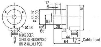
All dimension in mm with a tolerance of ±0.1mm
