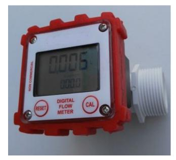
NXL developed and produced helical rotor flow sensor specially for Liquid dispensing industries, now a day water dispensing industries use plastic turbine flow sensor its k factor change with flow rate so for solution we developer helical rotor plastic flow sensor with same pulse k factor for full range also provide very good accuracy and repeatability in full range of measurement,
