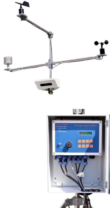
This Met Station is specially designed for Road weather monitoring applications. This system employs low power data logger system and rugged sensors for extreme road conditions. The system uses 12V operating voltage with a SLA battery backup while energy is harvested from a 12V/40W solar panel. Ethernet Interface is provided for Real time sensor monitoring. A stainless steel tripod stand is offered along with this system for robust mounting of data logger enclosure and sensors.
