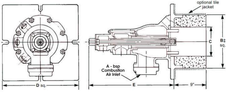
**NOTE:** For 6172-8, air and gas connections cannot be piped in the same plane because the "flower pot" type air connection flange would interfere with the  $2\frac{1}{2}$ " gas line.
