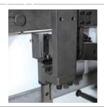
Stripping Bottom Frame guide: Adopt Taiwan famous linear guideway brand, instead of the traditional linear bearing and copper sleeve, which makes the stripping frame moves smooth, stable and greatly improve its service life, the service life of the linear guideway is 10 times of linear bearing or copper sleeve.
