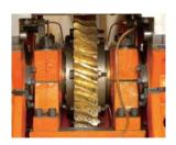
Main drive. The material of the worm gear use the high quality wear-resisting alloy copper, by the precision machine tool processing, the senior technician fine scraping, small wear and high precision High-frequency quenching treatment for crankshaft with chromium steel, long service life. The pendulum pole is cast by the ductile iron, high strength, wear-resisting durable.
