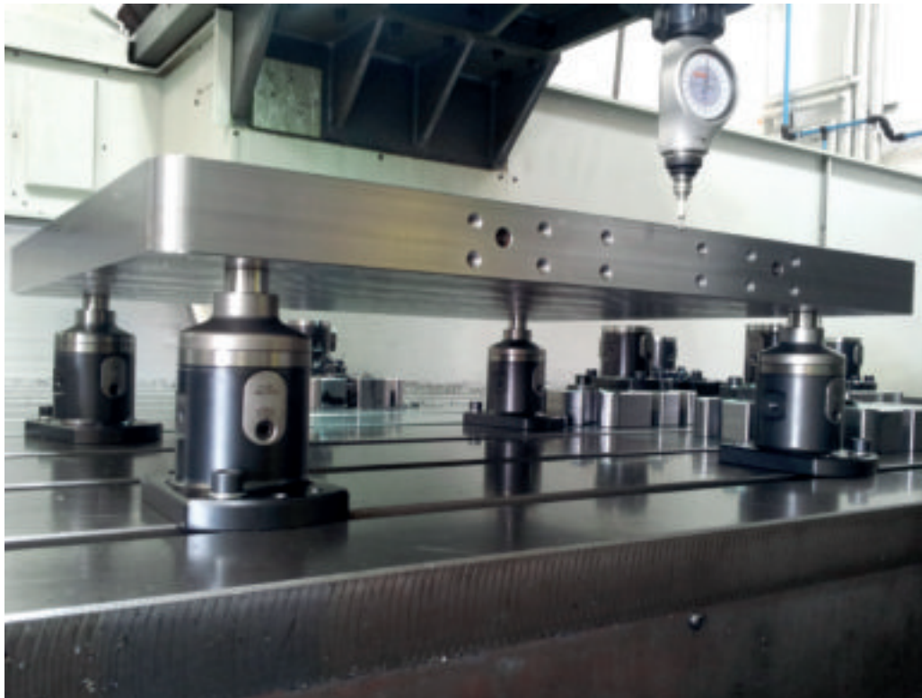
4 basic modules H=100 positioned directly on the machine table. The 4 reducers H=50 on top facilitate optimum access to workpieces. Clamping height 150 mm
