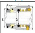
MAK-TECH SEALS manufacture and stock a 22/26mm step -balanced, 'O'-Ring mounted, robust single spring seal with positive drive from three drive studs on the coil base, to suit larger models of "SV- and e-SV-" series pumps.
