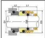
MAK-TECH SEALS manufacture and stock a 14mm MTS 131 seal to suit the reduced length seal chamber of various circulating pumps, such as "CE-" and "CO-" ranges with newer "A" suffix motors. The MTS 131 is the same dimensions to MAK-TECH SEALS MTS CS3, except for the reduced rotary working length.
