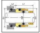
MAK-TECH SEALS manufactures a range of 'O'-Ring mounted conical spring seals to DIN "L1K" dimensions, to suit "FC-, FH-, SH-" series pumps.
