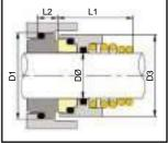
MAK-TECH SEALS manufacture and stock a range of 'O'-Ring mounted robust conical spring seals to DIN "L1K" dimensions, to suit "SV- and SVI-" series pumps. 12mm and 16mm also suit certain "e-SV-" series models
