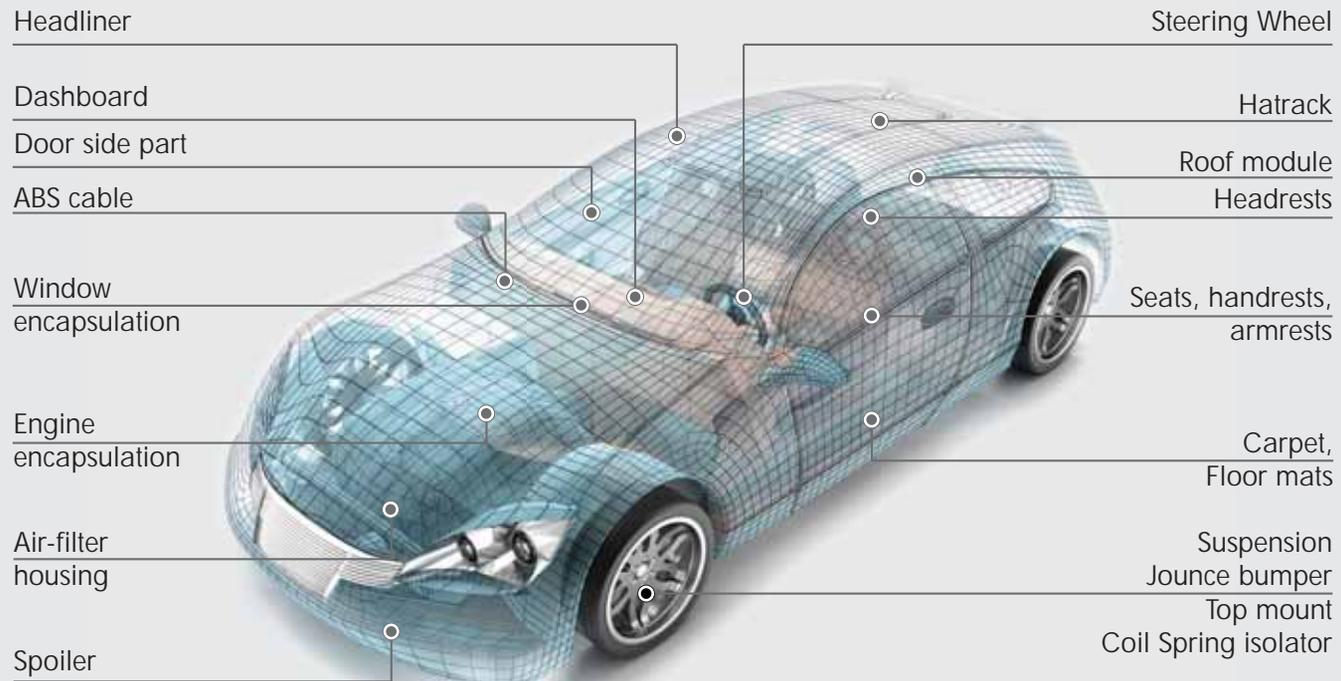
Polyurethane foam is an extremely versatile product used in countless applications worldwide. Polyurethane's mechanical properties can be isolated and manipulated through creative chemistry. This creates a number of unique opportunities to solve performance characteristics problems. It can have better hardness, better flexibility and better resistance .
