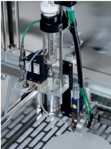
For substrates with a highly structured wafer topography, deep MEMS structures or a non-planar surface texture, the **iSPRAY-300** by SAWATEC ensures that the coating is as homogeneous as possible. It is a high-precision spray coater for manual spray coating or spray development processes and it is used specifically in research and development laboratories, for pilot productions and small production units in MEMS fabrication.
