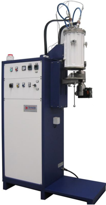
High Vacuum Furnace for 1.600°C Ø=40mm; HZH=70mm Equipment sold to: Universitat Autònoma de Barcelona - Spain
