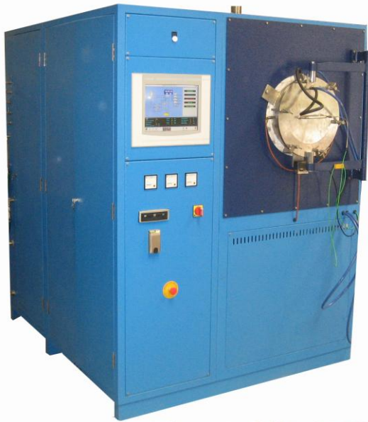
Debinding Furnace for 1.000 °C. Works with H 2 , N 2 , Ar, and Air. PC Panel for process control.
