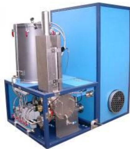
Model G4 with Debinding System Graphite furnace for 2.200°C Hot zone diameter: 200 mm Hot zone height: 300 mm Debinding system (condensation of the binders through trap and cold pot).
