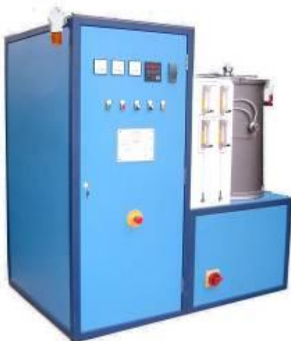
Model G4 with Debinding System Graphite furnace for 2.200°C Hot zone diameter: 200 mm Hot zone height: 300 mm Debinding system (condensation of the binders through trap and cold pot).
