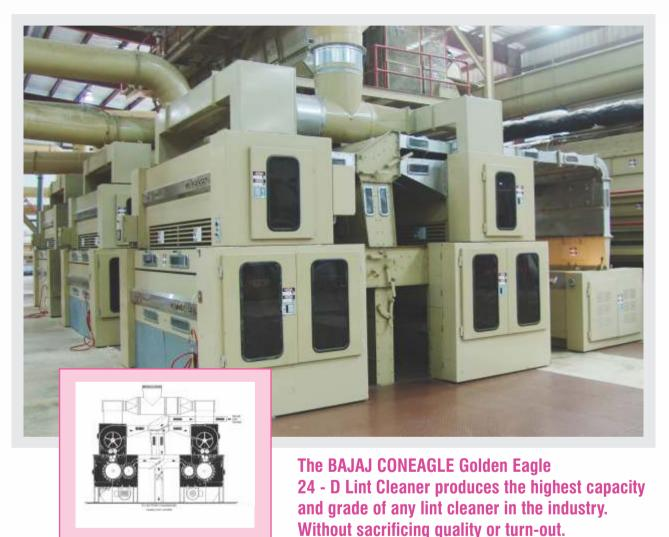
The BAJAJ CONEAGLE 24-D Golden Eagle Lint Cleaner is a saw-type, controlled-batt lint cleaner having two main assemblies, the lint cleaner base and the condenser assembly mounted on top of the lint cleaner base. One optional three-phase AC motor powers all drives in the condenser and lint cleaner.
