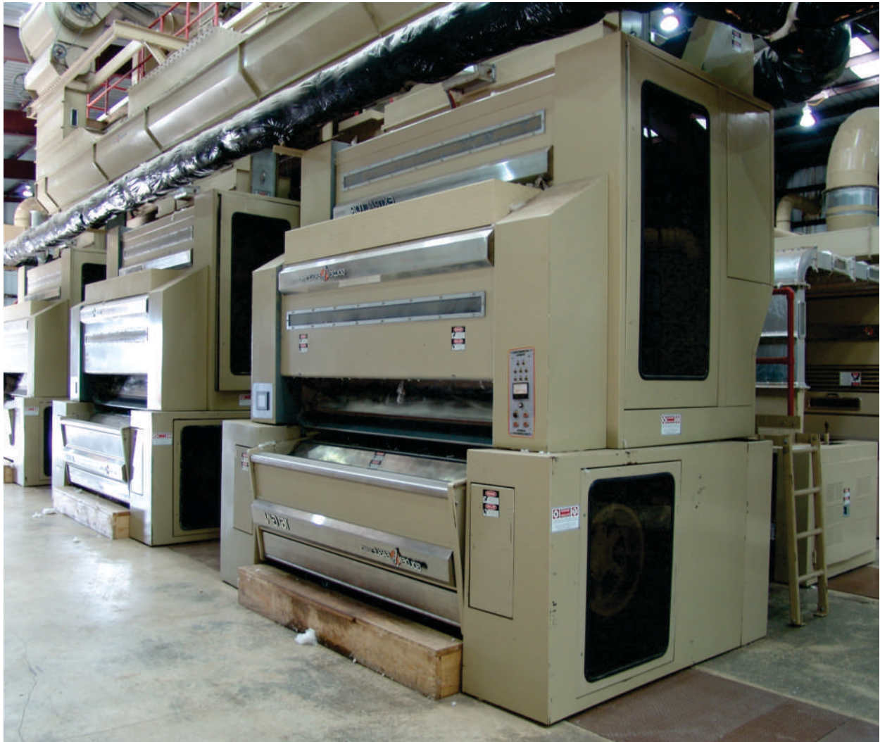
BAJAJ CONEAGLE Golden Eagle Feeder and BAJAJ CONEAGLE 161 Saw Gin
