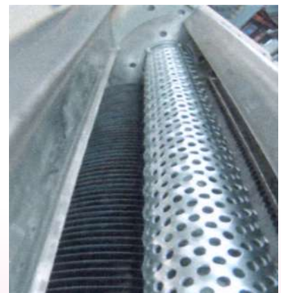
SEED ROLL CONVEYOR TUBE Seed is efficiently removed from the center of the seed roll.
