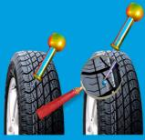
PunctureSafe covers more of the inner tyre at speed. When a puncture occurs, the centrifugal forces of the rotating tyre, plus internal pressure and escaping air, forces the PunctureSafe gel into the puncture and a permanent seal is created.
