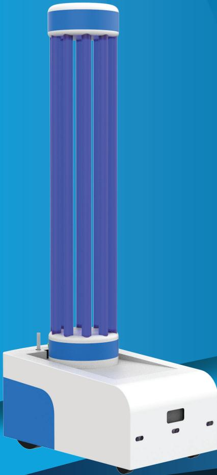
The Remotely operated robot is fitted with UV Disinfection Lamping system. These are operated remotely by an operator with the aid of Camera feedback. The trolley has a WiFi connected with a camera to get live Audio-Visuals of the path to the control station and interact along with the travel , announcing various messages.
