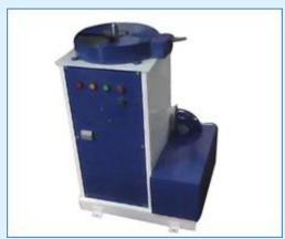
This machine is developed to get flat and parallel finish on the sample for high precision spectro-analysis. The blower casing and the dust collector are made integral with the main body which makes the machine compact and aesthetically superior. The rotating disc is dynamically balanced and mounted directly on the motor shaft instead of using belt, this ensures a uniform and noiseless operation.
