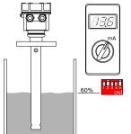
Total empty-fill of container is not necessary, any level can be calibrated using external multi-meter.
