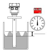
For liquid surfaces having turbulances, output damping time can be set from 0 to 120 seconds.
