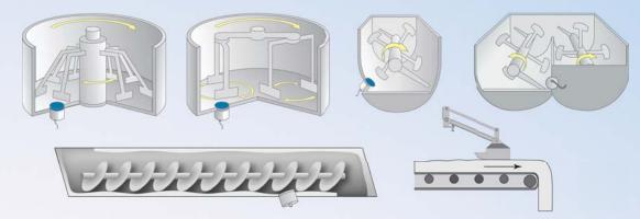
All types of static pan, horizontal shaft and ribbon mixer. Also suitable for installation in screw conveyors, chutes and other flush mount applications. For rotating pan mixers the Hydro-Probe Orbiter Sensor is recommended.
