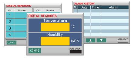
The Digital Readout Display displays online data for multiple channels. Single channel data can be viewed with bigger Digit size. The digit color channel changes when the alarming condition occurs. The alarms events can be viewed with date and time stamp in Alarm History screen. Display also shows the memory count which shows the status how more data samples can be stored in memory.
