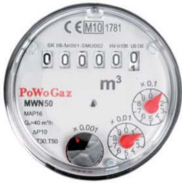
Roller-pointer counter housed, adapted for the radio module, it co-operates with NK and NO transmitters. The counter mechanism is equipped with the element of optical data transition is housed in the plastic airtight casing
