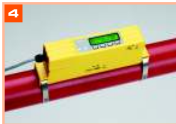
4 Click electronic assembly onto guide rail and sensor assembly
