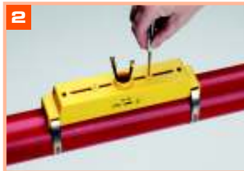
2 Clamp guide rail and sensor assembly to pipe and release sensor locking screws
