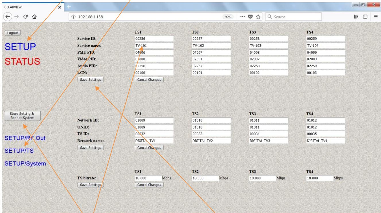
Set your **TS settings** for each channel then press **Save Settings** at the left-hand side. Once you have set all parameters and pressed Save Settings, finally press **Save Setting and Reboot System** to store permanently. The Bitrate setting must not exceed The allowable amount according to your modulator parameter settings. Please use the Chart below to determine the maximum bitrate value.
