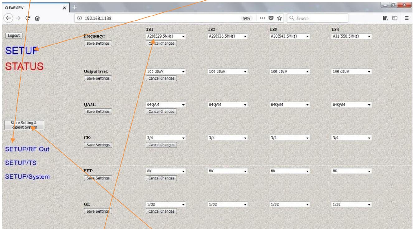
Set your channel **here** for each channel. Once set press the **Save Settings** button to the left. It is the same with Output Level, QAM, LCNs, CN, FFT and GI. After setting parameters and Saving, make sure you press '**Save Setting & Reboot System**' so settings are permanently stored.
