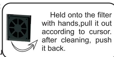
5. After using the machine for over 40 hours, please take off the dust filter and clean it (if have).
