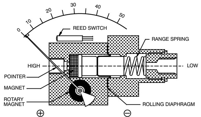
Model 200 DGR consists of a rolling diaphragm to sense the pressure difference. It can withstand maximum operating pressure up to 200 bar for all ranges. If pressure exceeds the rated maximum pressure, "O" rings & diaphragm inside the pressure chamber, will be damaged. If maximum operating pressure is within the allowable limit of 200 bar, but the differential pressure exceeds instrument range, there will be no damage to the instrument. Pointer will only go the extreme right end of the scale.
