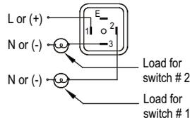
View of plug after removing the socket
