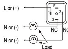
View of plug after removing the socket
