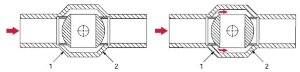
• Block and Bleed: cavity relief valve for over-pressure due to liquid thermal expansion.
