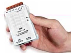
**1. Modbus TCP to RTU/ASCII Gateway application**
