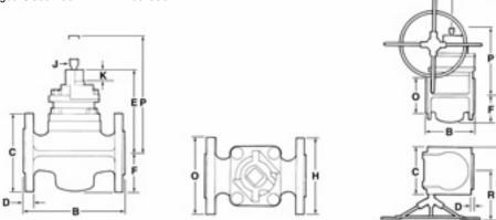
Flanged valves have face-to-face dimensions conforming to BS 5158 PN 10/16 & BS 2080 Class 150 Short, ANSI B16.10 & API 6D Class 150 Short. These valves are thus interchangeable with equivalent gate valves. Flanged valves have patterns conforming to BS 5353, BS 5158, ANSI B16.34, API 6D & API 599 Short (with steel plug).
