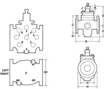
Valves have face-to-face dimensions conforming to BS 5158 PN 10/16, BS 2080 Class 150 Short, ANSI B16.10 & API 6D Class 150 Short. These valves are thus interchangeable with equivalent gate valves. Valves have Patterns conforming to BS 5353, BS 5158, API 6D & API 599 Short (with steel plug).
