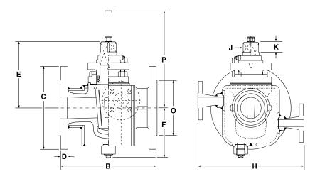
Valves have face-to-face dimensions conforming to BS 5158 PN 10/16, BS 2080 Class 150 Short, ANSI B16.10 & API 6D Class 150 Short. These valves are thus interchangeable with equivalent gate valves. Valves have Patterns conforming to BS 5353, BS 5158, API 6D & API 599 Short (with steel plug).
