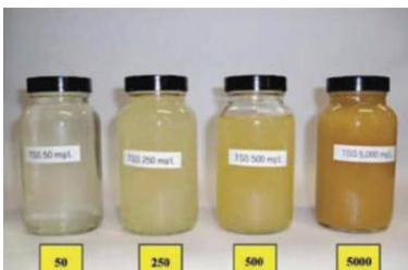
Water samples with various Total suspended Solids (TSS) Readings
