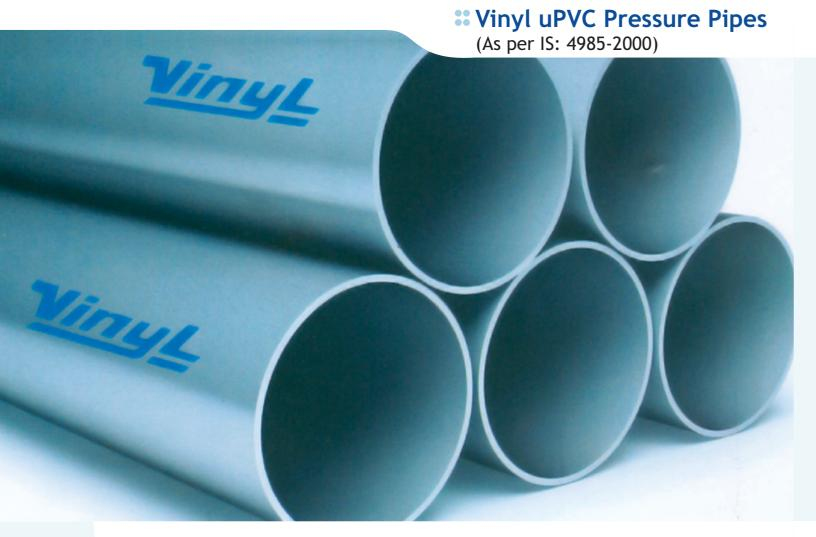
Vinyl uPVC Pipes Pressure & Non Pressure - are manufactured in accordance with IS:4985 covering a complete range from 20 mm to 315 mm. They are available in pressure ratings of 2.5, 4, 6, 8 & 10 kgf/sq. cm as defined in IS:4985. The pipes are provided with plain socket and suitable for solvent cement jointing and Bell end on request.
