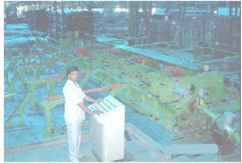
Hydro Tester , Make -Gallium Pressure Capacity - 250 Kg/mm 2 max
