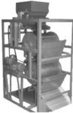
The Double Drum Machine is used for handling large capacities or difficult materials requiring more than one magnetic treatment. Double Drum Machines with individual jig shaker tray, can also be supplied. Triple Drum Machines can also be supplied if required.
