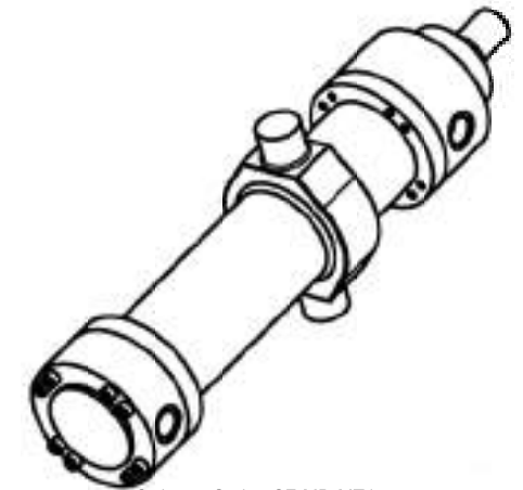
Ordering Code:- SF-MD-MT4 Intermediate Trunnion Mtg.
